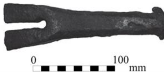
Figure 9. Wrecking bar with splayed head from repeated blows with a hammer.
